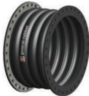
Style 1104 Quadruple (4) Wide Arch Rubber Expansion Joint with quadruple the movement and one-quarter the spring rate of style 1101. 36" ID X 24" FF shown.
