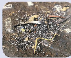
Foreign particles and sediment collected by screen gasket
