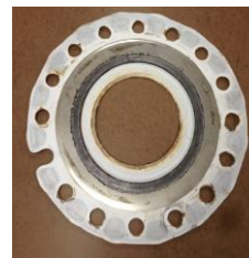
VSP's Fire Barrier PITA® Gasket after a four week production run.
