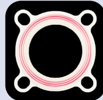
Pressure Film Highlights Concentrated Gasket Stress
