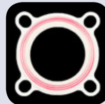
Pressure Film Highlights Gasket Stress
