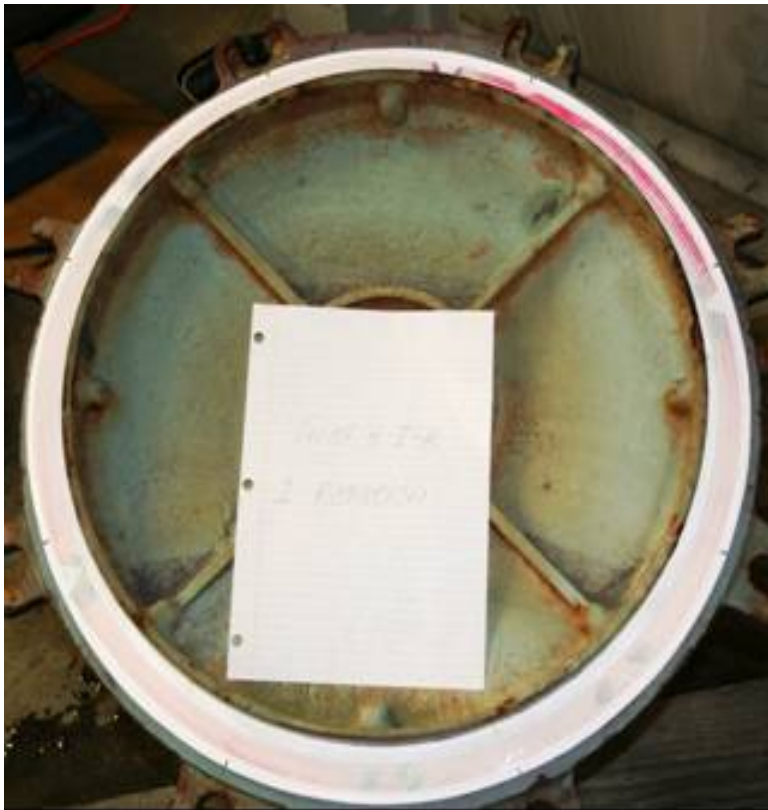
Lubricated Eyebolts 1 Pass Non-Uniform, Lower Overall Gasket Stress
