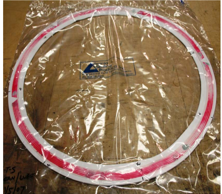
Cleaned & Lubricated Eyebolts More Uniform, Higher Overall Gasket Stress Developed
