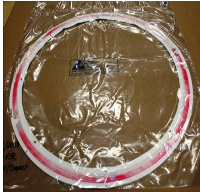
Lubricated Eyebolts w/Final Procedure More Uniform, Higher Overall Gasket Stress Developed
